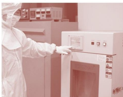
可编程恒温恒湿试验机 Constant Temperature and Humidity Test 测试胶片耐热性能、耐湿性能和耐候性能 Testing heat-resistance, humidity- resistance and weather-resistance
