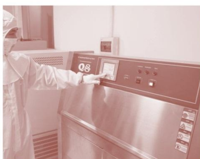
紫外线加速老化试验机 UV Radiation Accelerating Aging Tester 测试胶片的抗老化性能 Testing Aging-resistance
