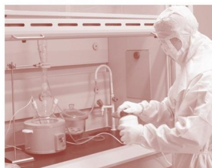
凝胶量检验设备 Inspection gel quantity equipment 测试胶片凝胶量 Test film gel quantity
